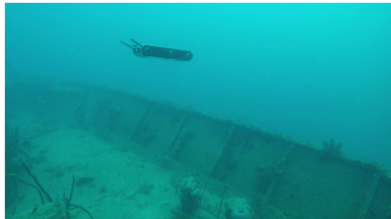
Fig. 1: Aqua2 AUV navigating over the Stavronikita shipwreck, Barbados. The front cameras are only seeing blue water when approaching the side of the wreck.
