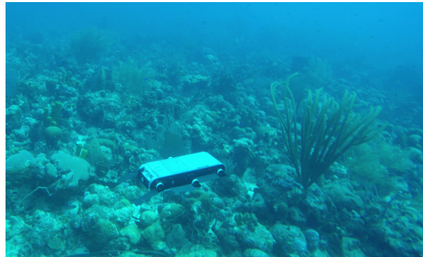
Fig. 1. Aqua2 vehicle navigating over a reef, collecting coral visual data.
